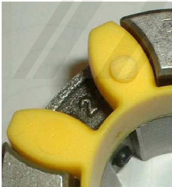
In Al-D hubs the set screw is located opposite the keyway, because the thread needs more engagement in aluminium than in steel or cast iron.
