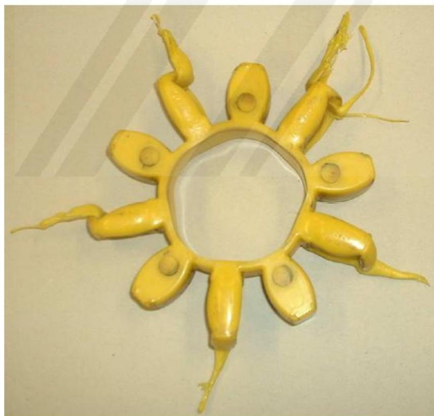
Vibrations can make The spider tooth melt From the inside. This melting process creates internal pressure inside the spider tooth. The head of the spider pops open and the liquid PUR material gets out. The material wraps around the coupling and „freezes“. It looks like Spaghetti.
